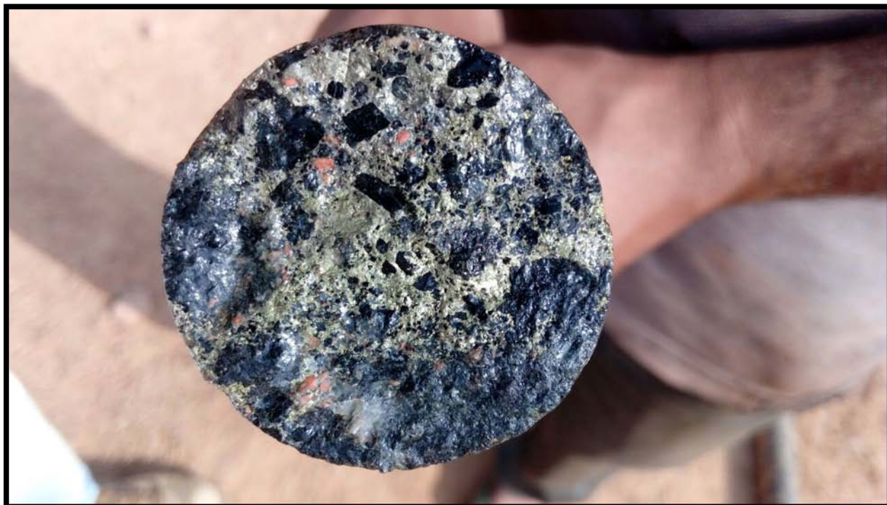
Photographs of the sulphide zone encountered in the BH No.-MNI-02 in Kanawat-Chala -Karath-Bagholi area, (WR-RAJ-07), District Jhunjhunu & Sikar, Rajasthan
