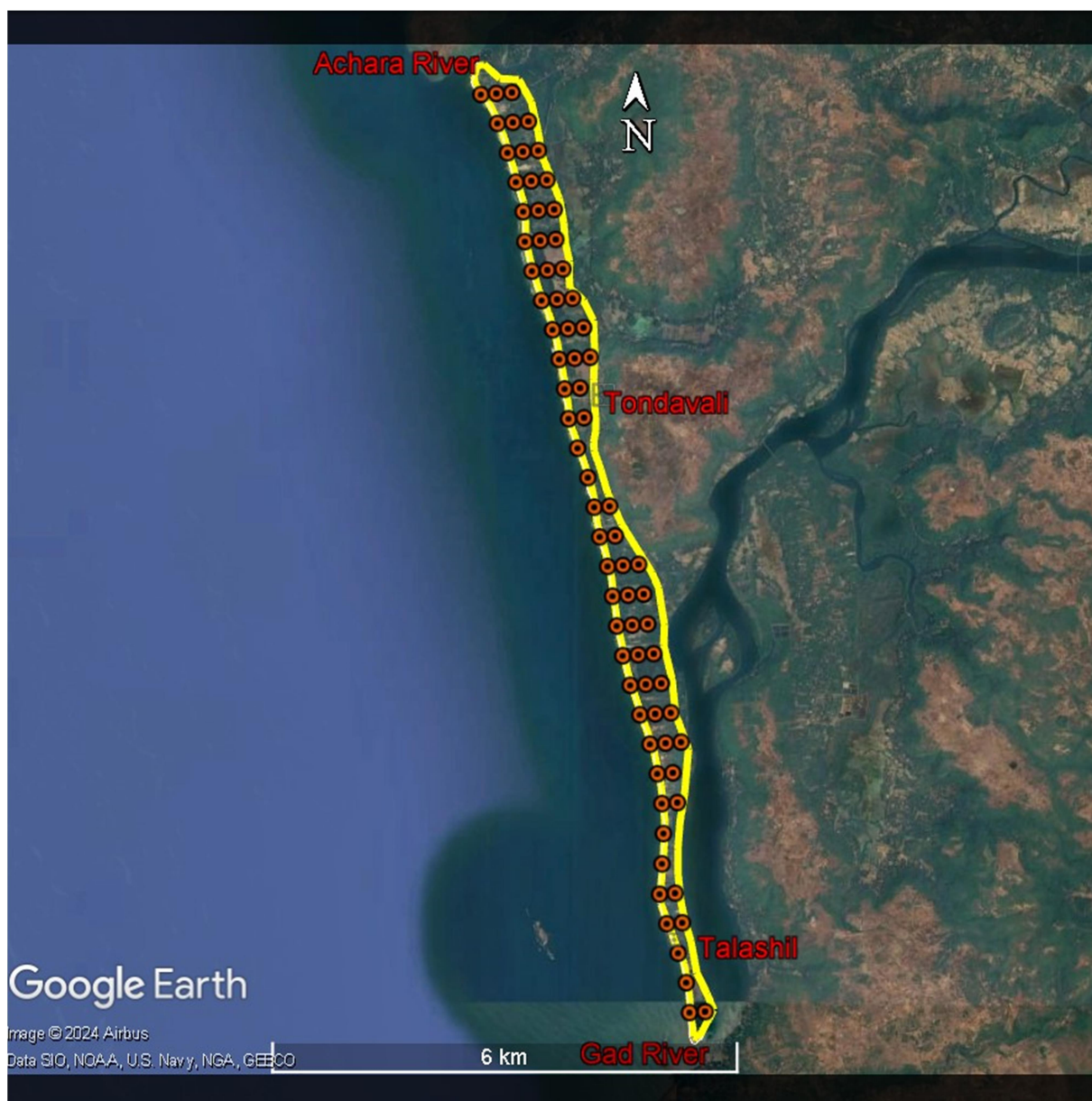
Fig.3A: Proposed Sampling Point locations (75 Auger Borehole) at 400m x 200Grid size over Google earth imagery
